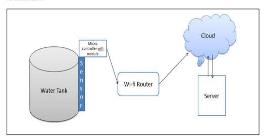
Fig.1 Architecture of Water Level Monitoring System
