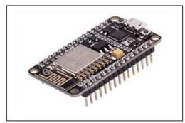
Fig. 4 Wi-Fi Trans-receiver
